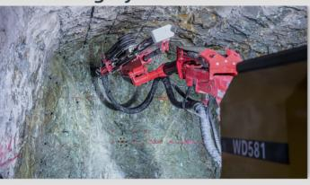
Adopting high efficient and fast electro-proportional hydraulic control drilling system, including automatic drilling, automatic retraction, automatic release of jamming brazier and other functions.
